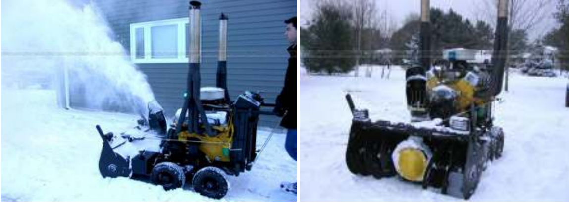
At last, a solution to our heavy, wet snow! Kai Grundt, a resident of Northern Ontario, built this snowblower. It is propelled by a 454 Chevy V8 which churns out 412 HP and 430 Lbs Ft of torque.
