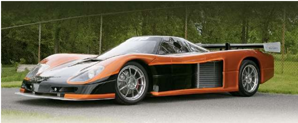
Another rare one. This is a Chevrolet Corvette GTP. It’s not really a Corvette at all, but is a collaborative effort between General Motors and Lola Cars International in England. Its purpose was to permit GM to compete in the IMSA GT Championships from 1984 to 1989. Lola built the chassis, and GM put on the body. The car was powered either by a turbocharged 3.4 litre V6 or by a normally aspirated small block V8. *****
